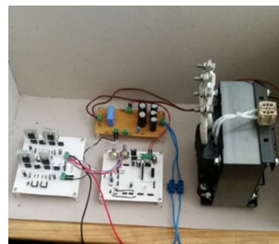
Figure 4. Single-phase inverter system
